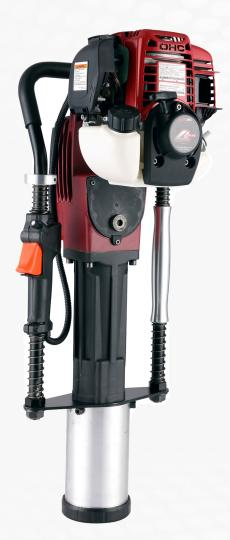
The DFS Post Pounder uses a 2 stroke 52CC gasoline engine that has the power you need to drive your pipe into the ground. Built for durability and power, this versatile post pounder will not only handle the galvanized steel pipe for a vinyl fence but it also accommodates other sizes of posts and pipe. The sleeve adaptors that are included are 2", 2.75", and 4".
